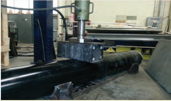
Crush Test on Concrete Filled Pile
