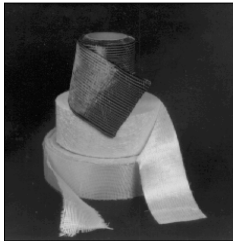
Woven/stitched goods increase transverse properties of pultruded profiles.
