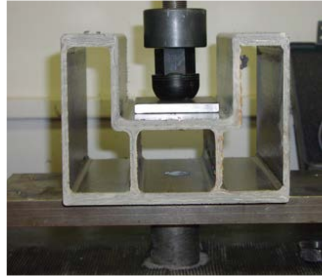
Figure 1. Photo of the Tie-rod push through test conducted in CCG Lab.
